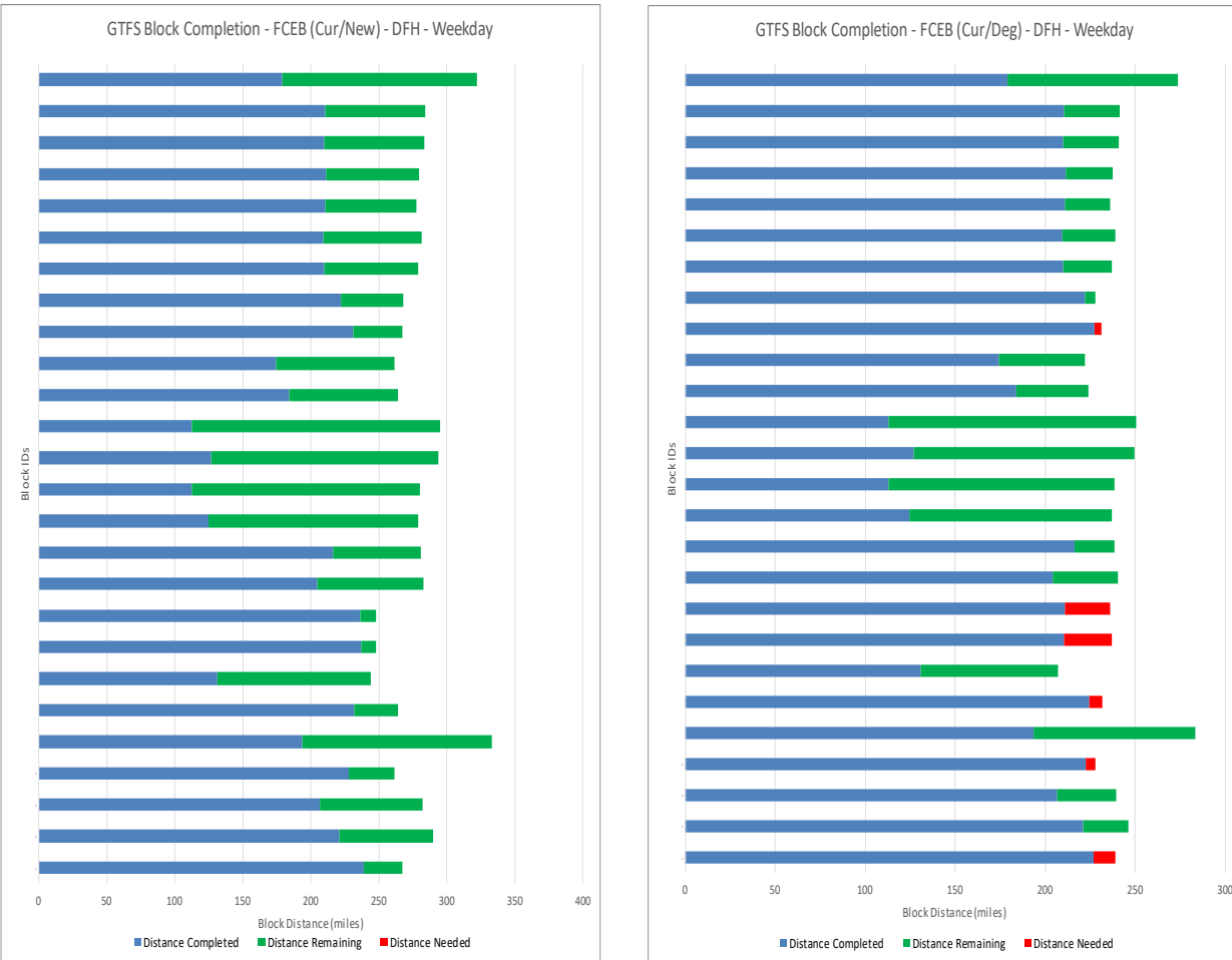
Figure A-3: Block Completion for All Blocks using (a) New and (b) Degraded 40-ft FCEB in Winter with DFH
